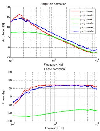
Fig. 4. Amplitude correction characteristics (top graph) and phase correction characteristics (botoom graph) for each particle velocity signals.
