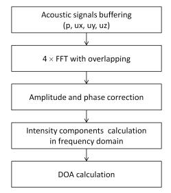
Fig. 3. The block diagram of the algorithm applied for the sound intensity determination.
