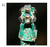
Fig. 2. 3D SIP in different orientations, all microphones are visible.
