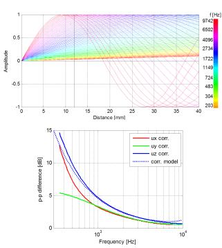
Fig. 1. Distribution of amplitude as a function of the distance between microphones, a black vertical line indicates a 12 mm distance, as is in the developed sound intensity probe.
