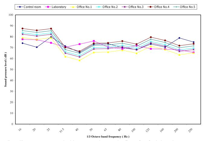
Fig. 3. The noise spectra measured at laboratory, control rooms and 5 offices in Cairo South electrical power station.
