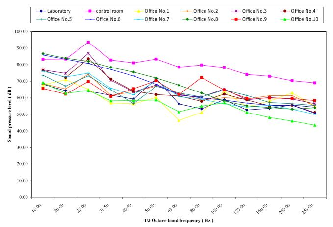
Fig. 1. The noise spectra measured at laboratory, control room and 10 offices in Shopra Elkhiema electrical power station.
