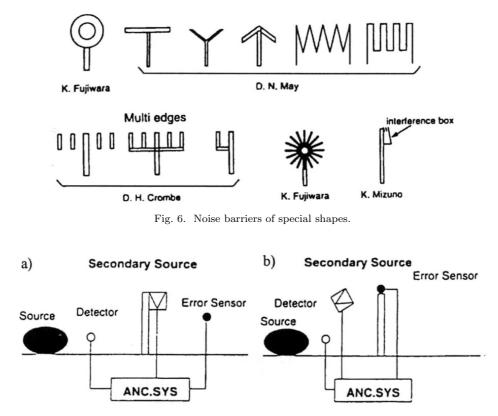
Fig. 7. Experiments of active noise barrier; a) S. ISE et al., b) A. OMOTO et al.
