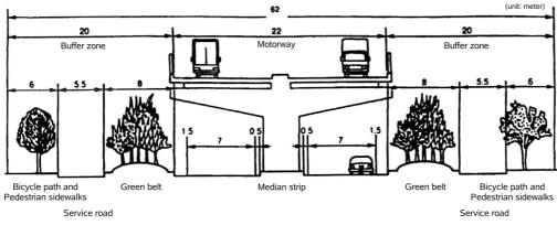
Fig. 8. Highway with buffer zone (Tokyo Outer Ring Road).
