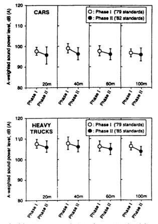
Fig. 3. Sound power level (maximum at pass-by 7.5 m from a microphone) from accelerating vehicles measured at different distances from a stoplight. Cars in the left part and heavy trucks in the right part of the figure [1].
