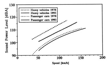
Fig. 4. Change in sound power levels of Japanese vehicles 1978–93, as measered in a tunnel [1, 2].
