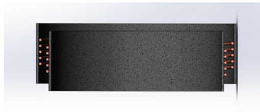
Figure 5. Schematic diagram of the shaft coupler coil offset 5mm
