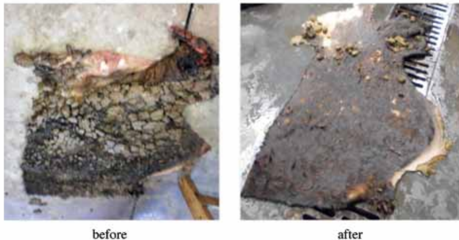
Hide sample with numerous adobe type manure before and after presoaking in formulation composed of 25% Std SF + 1% Sodium Carbonate + 5% Crude Glycerol + 0.025% Cellulase + 0.025% Xylanase + 1% NaOH
