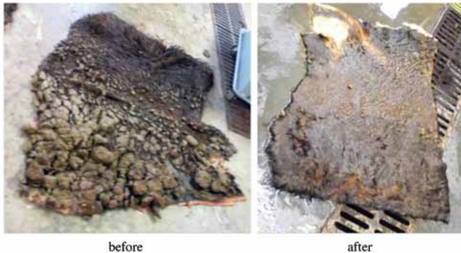
Hide sample with numerous adobe type manure before and after presoaking in formulation composed of 25% Std SF + 5% Crude Glycerol 2% NaOH + 1% Sodium Percarbonate + 0.15% alkaline protease (pH 13.4)
