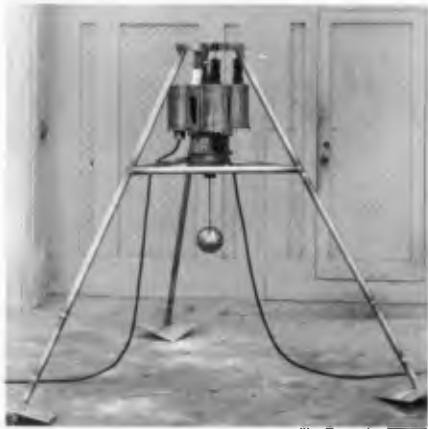
Fig. 8. Current meter mounted in leveling tripod.
