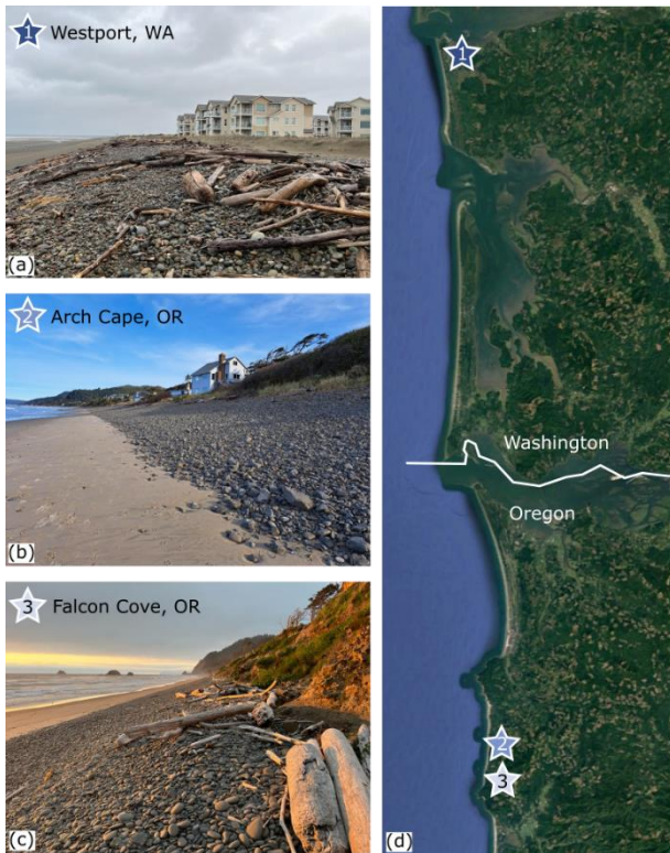
Figure 1 - Map and photos of project sites. (a) Westport, Washington is an engineered dynamic revetment constructed in January 2021. (b) Arch Cape, Oregon is a natural composite beach with subangular cobble. (c) Falcon Cove is a natural composite beach with rounded cobble. (d) A map of the project site locations.
