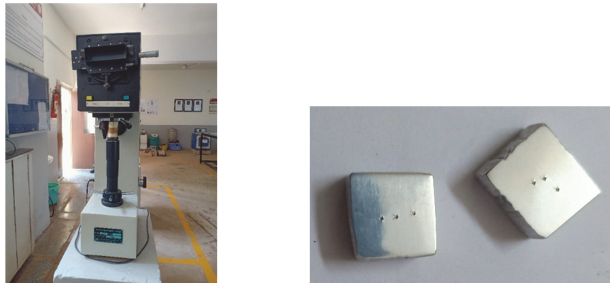
Figure 6: Vickers hardness tester and Hardness specimen.
