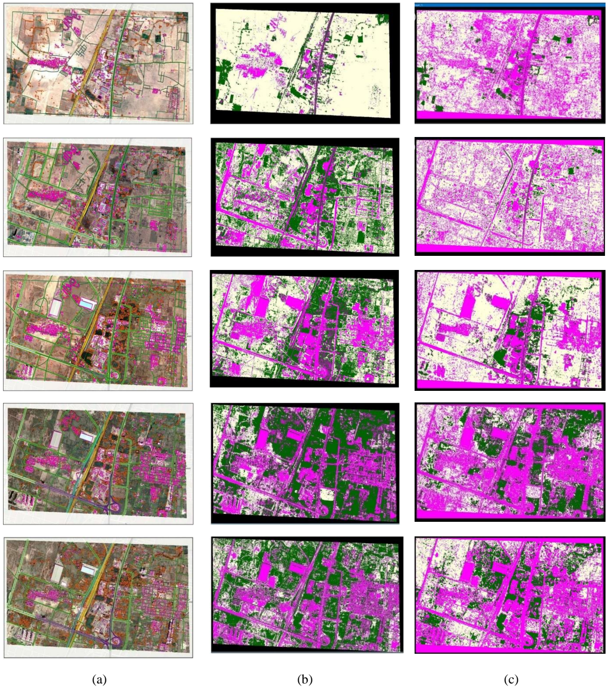
Figure 6. Row wise:- Row 1: Year 2005, Row 2:Year 2010, Row 3: Year 2015, Row 4:Year 2020, Row 5: Year 2023; Column wise:- (a) Interpretation of Satellite Data, (b) Unsupervised Classification Result, (c) Supervised Classification Result.
