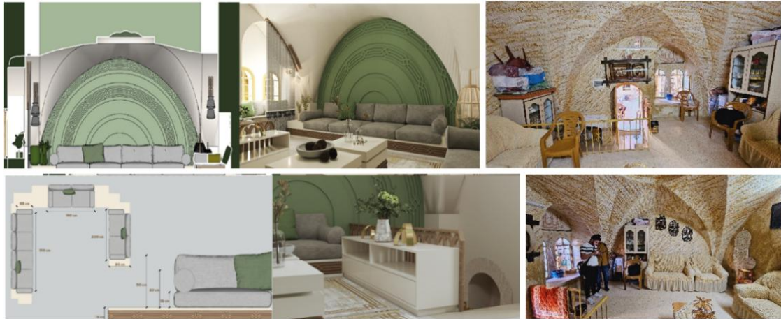
Figure 8: Presents a comparison between the current condition of a room in Al-Rajabi House and the proposed design interventions aimed at enhancing its functionality and preserving its heritage features. (Source: by the author, 2023).
