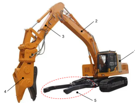
1-Scrap car dismantler 2-Boom 3-Arm 4-Hydraulic clamp 5-Working arm
