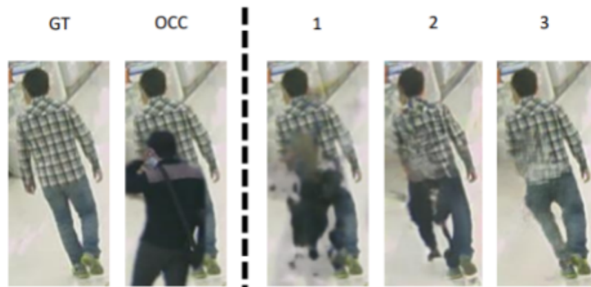
Figure 2.11: GANs are providing a method to reconstruct hidden images of people and objects. Images 1–3 show reconstructions as compared to an input occluded image (OCC) and a ground truth image (GT) (from Fulgeri et al. 2019, fig. 6).
