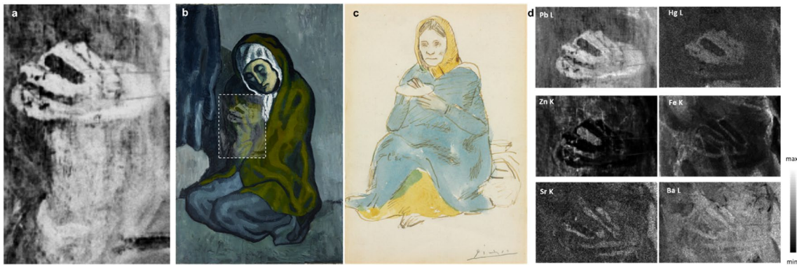
Fig. 4 a Detail Pb L map (step size 1 \times 1 \text{ mm}^2 —area 120 \times 230 \text{ mm}^2 ) acquired in area highlighted in b ; b Visible picture (© of the reproductions of works by Pablo Picasso: Pablo Picasso's Estate. VEGAP. Madrid, 2020. Permission to reproduce courtesy of VEGAP) overlapped with Pb L map; c privately owned watercolor from Picasso dated from the same period; d MA-XRF Pb L, Hg L, Zn K, Fe K, Sr K and Ba L maps (step size 1 \times 1 \text{ mm}^2 —area 150 \times 100 \text{ mm}^2 )
