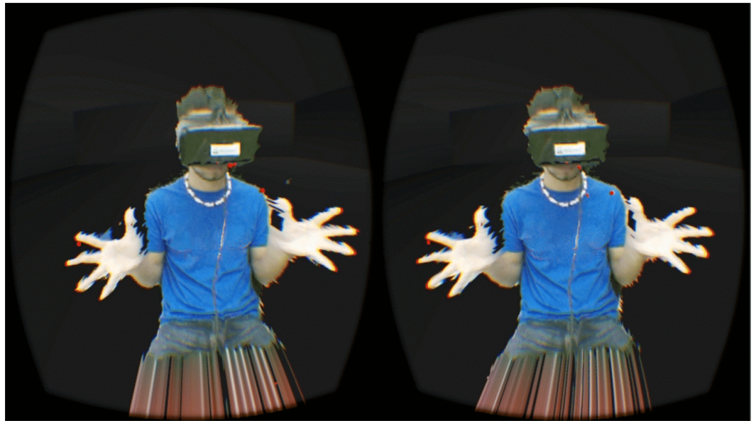
Figure 5 Avatar visualization with polygon surface. Similarly to Fig. 4 we see both left and right frames projected through the Oculus Rift's lenses. In this case, the avatar has a continuous surface, except for its borders and generated artifacts on the base. The red dots that represent Kinect joints can still be noticed behind the avatar and its right index finger.
