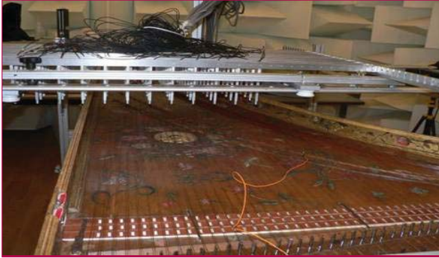
Fig. 6 - Acoustic holograph of the J. Couchet harpsichord The microphone grid is placed over the instrument at a precisely known distance. The experimental setup avoids any contact with the instrument and the experimental conditions are easily reproducible. Measures are performed yearly. A difference in the measurements would indicate an evolution of the vibrating structure and would result in a reassessment of the conservation conditions. Photo: S. Leconte © Cité de la Musique
