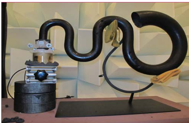
Fig. 4 - Acoustic impedance experimental setup Measure of the acoustic impedance of a serpent. The impedance head is placed on the upper extremity of the instrument (on the left of the figure). The acoustic impedance characterizes the "resistance" of the material to the passage of sound. It is defined as the ratio of sound to particle velocity and is frequency dependent.
