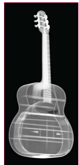
Fig. 5 - Radiography Radiograph of a "Selmer" jazz guitar. All the internal components are perfectly distinguishable, in particular the double resonator system, patented by Mario Maccaferri who was responsible for the guitar fabrication in the company. A weakness, detached adhesives, or a fracture would be immediately discernible. Photo : S. Vaidelich© Cité de la Musique
