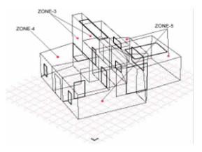
Figure 8. Location of thermal zones 3-4-5 of ground floor.
