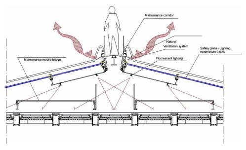
Figure 11. Detailed section of the external structure of the main skylight.
