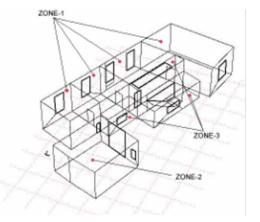
Figure 7. Location of thermal zones 1-2-3 of first floor.
