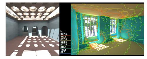
Figure 9. Examples of Radiance simulation.
