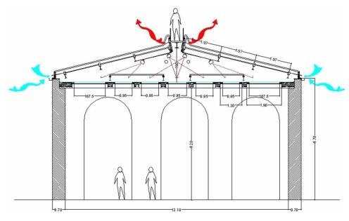
Figure 10. Project section of one of the skylights.
