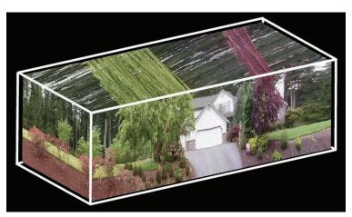
${\bf 3}\,$  Video cube captured by driving a car down a residential street with a camera pointed out the window.
