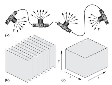
**2** (a) A camera moves along a path and captures light rays. (b) Stacking the images one on top of another yields (c) an *x*-*y*-*t* video cube. Each slice of the video cube produces a path image and represents a subset of the captured light rays (shown figuratively in red).
