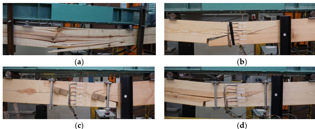
Figure 15. Failure views for selected beams (a) A01, (b) E03, (c) F01, (d) G02.
