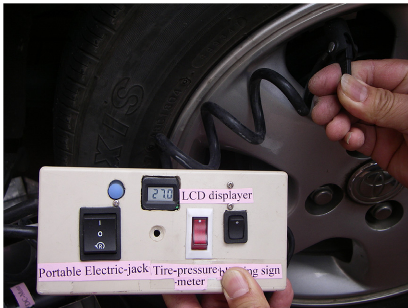
Fig. 6. Real photograph of the ICRT measures and stabilizes the Tire-pressure efficiently.
