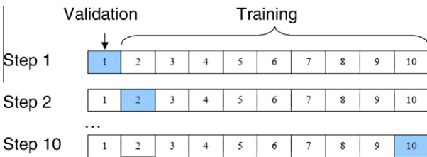
Fig. 13. k-fold cross-validation using k = 10.
