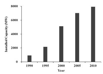
Figure 3. Installed capacity of CHP system in Taiwan during the 1990–2010 period.
