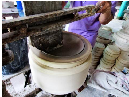
Fig. 2. A jigging machine used in this study
