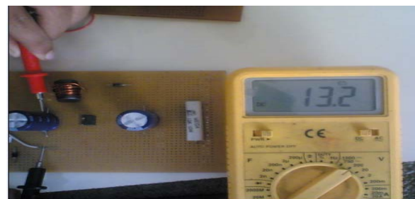
Fig. 4d. Display of the input voltage
