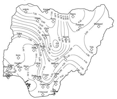
Figure 2. Nigeria wind map in m/s determined from 40 year's measurements at 10m height, obtained from Nigeria Meteorological Department, Oshodi, Lagos State, Nigeria (NIMET) [23]
