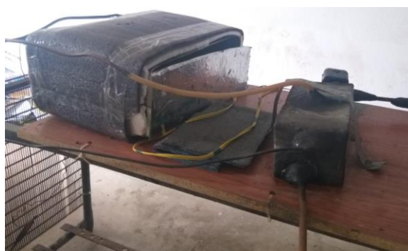
Fig.3:-Condenser, evaporator and absorber unit
