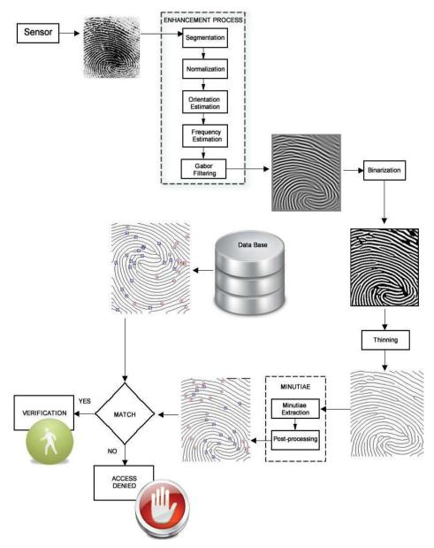
Fig. 1. Fingerprint authentication system
