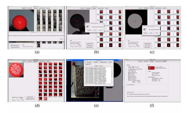
**Figure 33:** User interfaces of the PTMbuilder at Museum D. Diogo de Sousa: (a) attempt to locate the ball, (b) black ball detection and tuning, (c) red ball detection and tuning, (d) highlight detection and tuning, (e) HLT/LP file edit over PTMviewer, and (f) User options interface.
