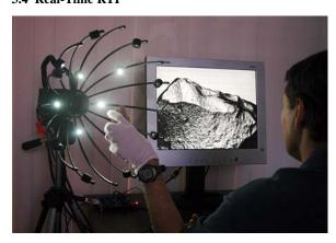
**Figure 10:** Real-time surface detail enhancement is possible using high brightness L.E.D.s coupled to a high speed camera and GPU.
