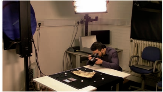
Fig. 4 Kazim Pal undertaking the digitization process, which required much movement around each folio. You can also see here a set of small ceramic balls placed around the folio which we originally had planned to use for calibration: these were not required as our work progressed but they remain in the capture shots. Video 1 (which is available in the online version of this paper) shows a time-lapse of a typical capture sequence, indicating the range of angles required to gain a complete coverage of each folio side, and indicating that the digitization process was non-contact
