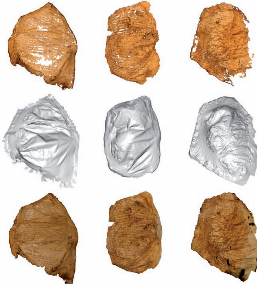
Fig. 7 Top: Dense point clouds generated by VisualSFM and PMVS. Middle: Triangle meshes generated by applying Poisson Surface Reconstruction to the point clouds. Bottom: Textured meshes generated by back-projecting and blending the original images
