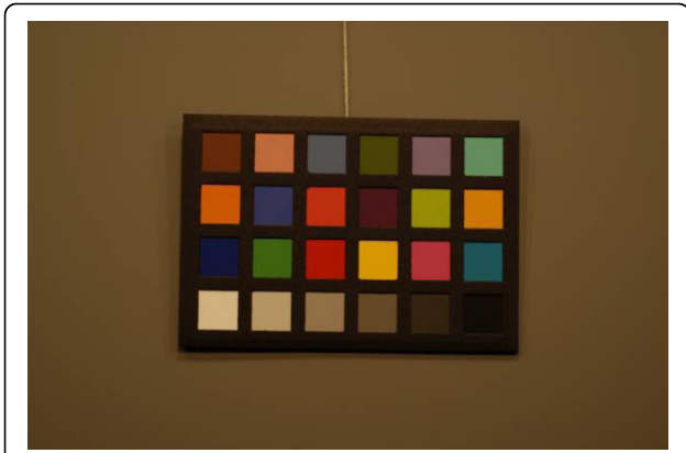
Figure 4 Example with Nikon D200: MBCC under illuminant A (3000 K). Camera: exposure bias -1, automatic white balance.
