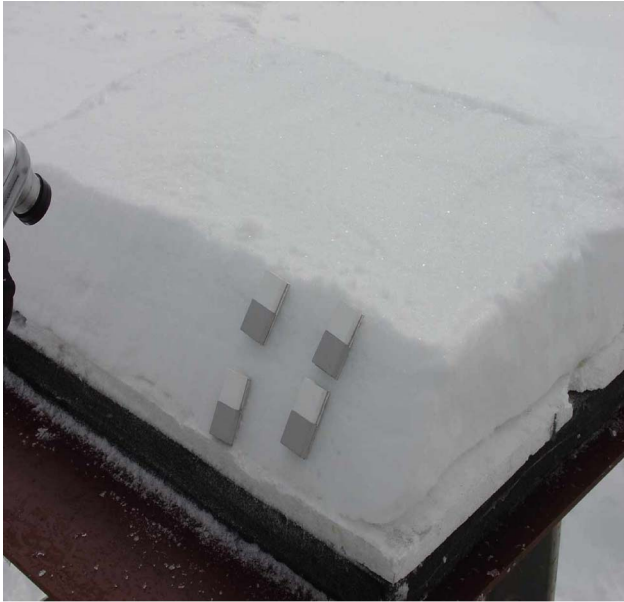
Fig. 2. (Color online) Preparation of the snow slab for the NIR photography. Four gray-white targets are placed on a smoothed snow side.
