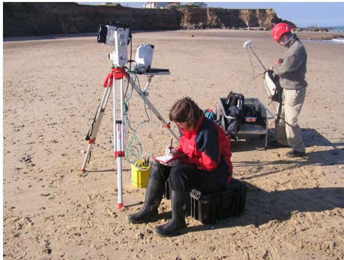
Figure 1 Laser scanner mounted on tripod – mobile set-up
