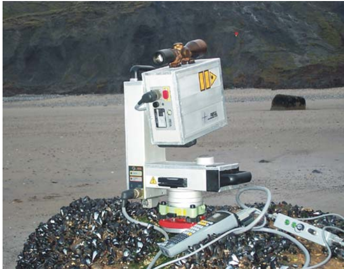
Figure 4 Laser scanner mounted to rock-bolt on WW2 concrete block – temporary set-up
