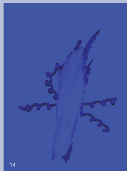
Figs 11-15 The pixels are only capable of measuring the dark and bright parts of an image, and in effect are only capable of producing a black and white image (Fig. 11). Colour is created by the three channels red (Fig. 12), green (Fig. 13) and blue (Fig. 14), and combining these channels produces a colour image (Fig. 15)
