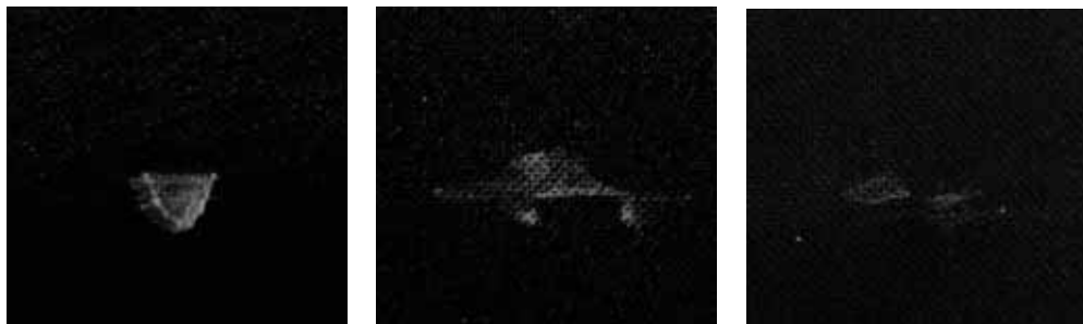
Fig. 2. Dry-swabs of stainless-steel sample area contaminated by Ibalgin® suspension (a) 500 \mu\text{g.dm}^{-2} ; (b) 300 \mu\text{g.dm}^{-2} ; (c) 75 \mu\text{g.dm}^{-2}
