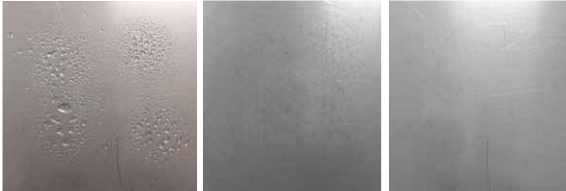
Fig. 1. (a) spraying the contaminant solution on model surface area; (b) surface contaminated by 500 \mu\text{g.dm}^{-2} caffeine; (c) surface contaminated by 75 \mu\text{g.dm}^{-2} caffeine
