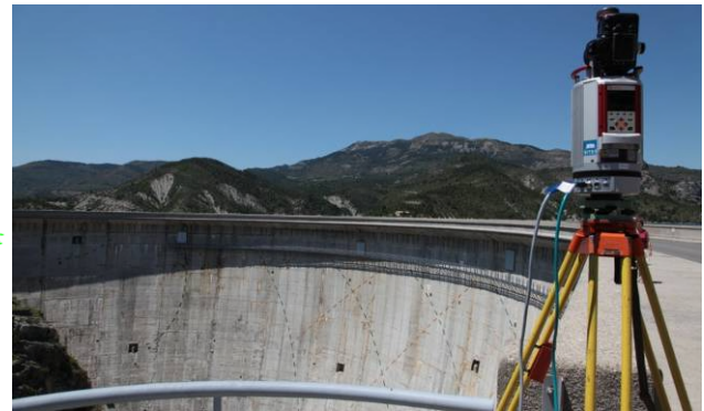
Figure 4. LIDAR in operation on the left bank of a dam
