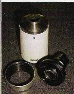
Picture 2: (Left) Nikon MDC relay lens (part number 82014). The small ring located on the left side of this picture had to be removed. The field of view (or field number) of this lens is 18 mm.
