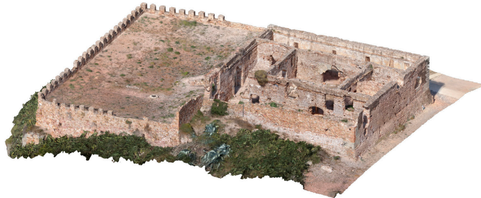
Fig.1 3D model obtained by SfM photogrammetry. Terrestrial and aerial pictures.
