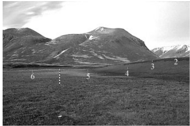
Fig. 2. The automatic digital photograph from the ZERO-CALM2 grid in the Zackenberg area, 18 August 1998, with measuring sticks located at vegetation limits in a transect through the snowpatch site. The photographed transect is about 100 m long. The distance from the camera to sticks 2–6 varies from 65 m to 105 m. The stick in the foreground, with 10 cm intervals, is only 15 m from the camera. The photograph is taken towards the northwest. Seen in the background are the southeast side of the Zackenberg mountain, reaching 1360 m a.s.l., and, to the right, further distant parts of the Dombjerg mountain (1300 m a.s.l.).
