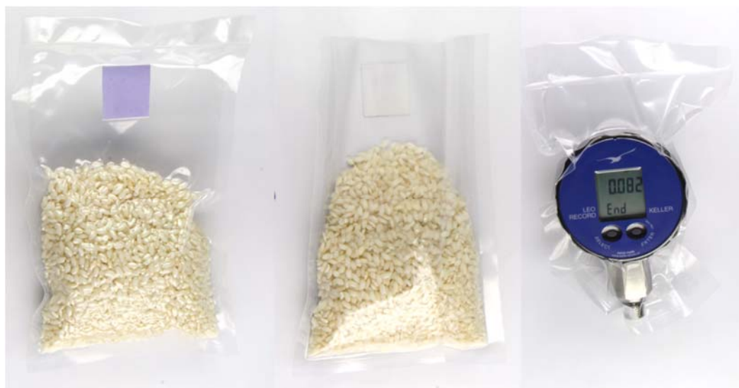
Fig. 4: Digital photograph of the vacuum packed risotto rice with OCP indicator, before (left) and after opening (middle), and vacuum packed digital vacuum meter.
