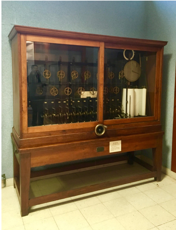
Bidston-Kelvin tide prediction machine, built in Glasgow in 1925. Photograph taken by H. M. Rawsthorne at SHOM, Brest, on 18/12/2018; licensed under CC BY 4.0.
