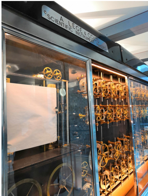
Doodson-Légé tide prediction machine, built in London in 1950. Photograph taken by H. M. Rawsthorne at NOC, Liverpool, on 15/01/2019; licensed under CC BY 4.0.
