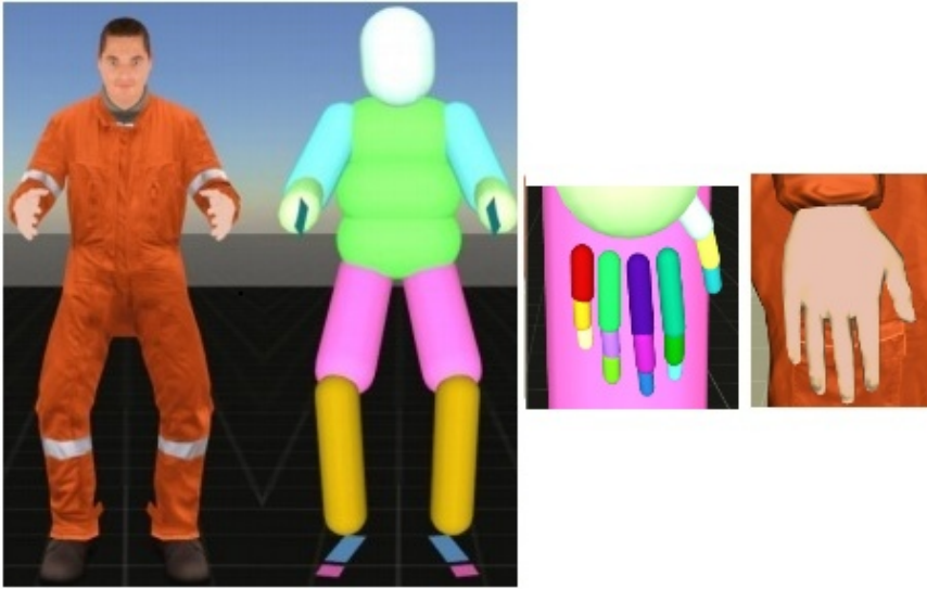
Fig. 2: DHM with skinning and collision geometry (left). Right hand model with skinning and collision geometry (right)
