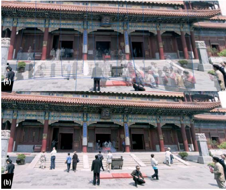
Figure 7. Panoramic composite. (a) The overlapping images are aligned and blended together, resulting in ghosted figures; (b) graph cut finds regions in each image to stitch together to create a consistent scene.
