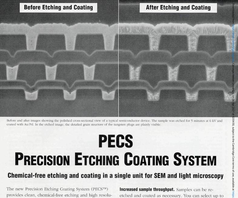
Before and after images showing the polished cross-sectional view of a typical semiconductor device. The sample was etched for 5 minutes at 6 kV and coated with Au/Pd. In the etched image, the detailed grain structure of the tungsten plugs are plainly visible.
