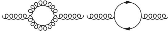
FIGURE 1.3: Virtual corrections to the gluon propagator: gluon loop (left) and fermion loop (right).
